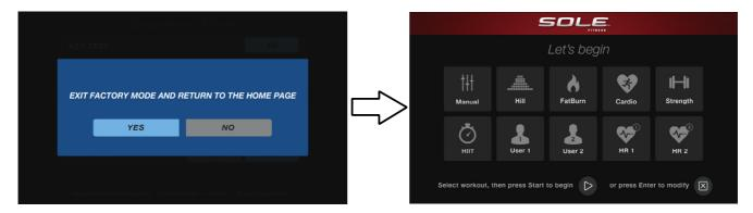
**Incline Calibration:** If there is a problem with the incline, try running the calibration. Press the Incline up key and the Start key at the same time. Hold them down for 5 seconds and press Start key to begin Incline calibration will start and run automatically. Exit the calibration page you need to power off then power on. If the problem persists contact service department.
